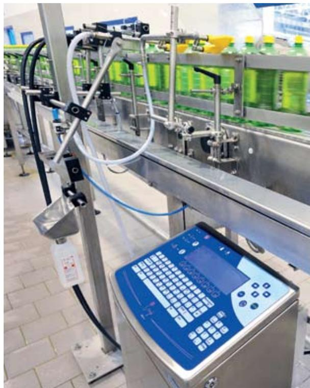
**The 9040 IP65 prints two lines of codes on each bottle with 11 to 13 characters: the plant initial, the production line number and the bottling date and time.**
